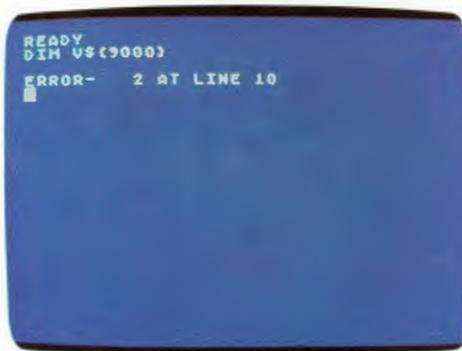
The computer is telling you there is a mistake in program line #10. You must go back to that line, find the mistake, and make the correction.
