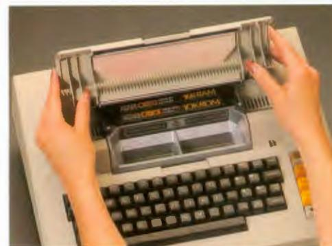
**4** Position your new memory module directly behind the existing 16K RAM module and push it firmly into place.
