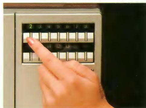
**7** Set the Channel Select Switch on the right side of the computer console to the same channel. After you turn on the computer, you may need to adjust the fine-tuning knob on your TV to improve the reception.
