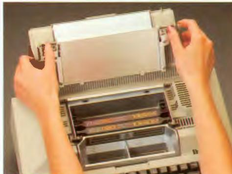
**6** When the cover is in place, press down on it with one hand, and move the latches back into the locking position with the other hand. If the latches do not lock without force, remove and reposition the cover.
