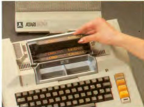
**5** Place the cover back into position, making sure you match up the notches on the lower back section of the cover and the cover housing.
