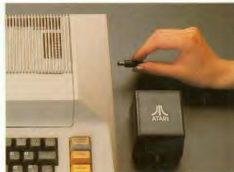
**10** You are now ready to turn on your computer. Make sure the cartridge door is closed. The main power switch, labeled **POWER ON/OFF**, is located on the right side panel of the computer. As soon as you move the switch to **ON** (and assuming you have not inserted the ATARI BASIC cartridge), the words ATARI COMPUTER-MEMO PAD appear on your TV screen. Whatever you type will also be displayed on the screen.
