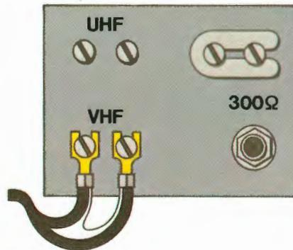
If it looks like this, loosen the screws holding the U-shaped slider and move it to the position on the switch box marked 300 OHM (or 300 $\Omega$ ).
