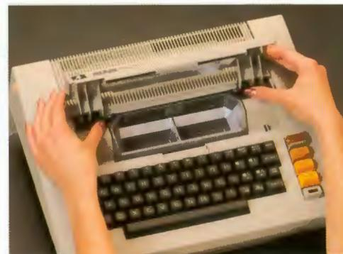
**3** Carefully remove the ribbed cover from the computer. You will see a 10K ROM module and one 16K RAM module already inserted.
