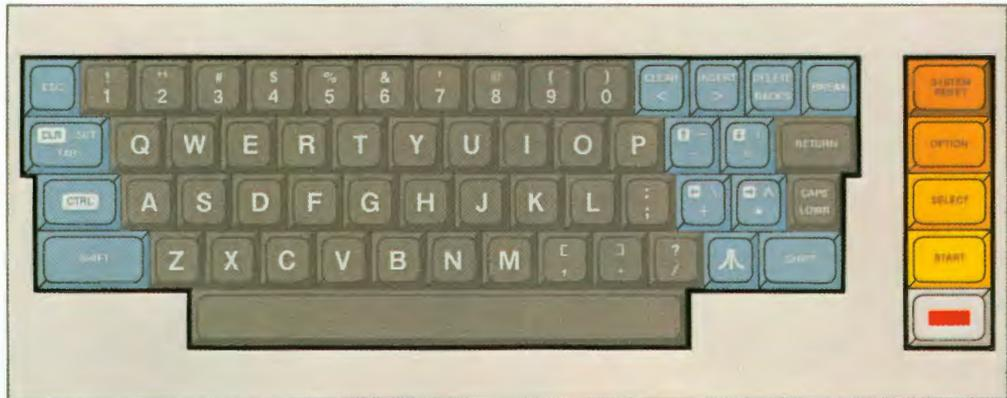
The **ESC** (ESCAPE) key function depends on the application with which you are working. For instance, if you are writing programs, the **ESC** key disables the cursor control movements and prints a graphics character instead. Or, if you are working with the ATARI Word Processor and are in the edit mode, pressing **ESC** takes you out of the edit mode.
