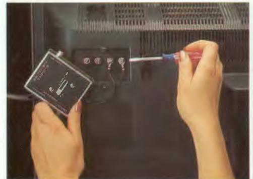
**3** Peel off the protective cover sheet from the self-adhesive square on the switch box and press the switch box onto the back of your television so it adheres to the casing.
