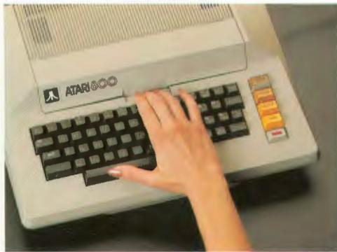
**2** Insert the cartridge into the left slot with the label facing you. Press down on the cartridge gently, but firmly, until the cartridge is in place.
