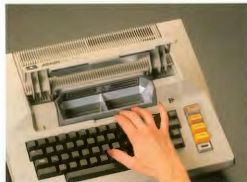
**2** Rotate the black latches located above the cartridge slot in the direction of the arrows as shown.
