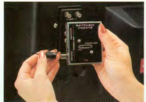
**2** Now locate the short, twin-lead cable marked **TV** that comes from the TV Switch Box and connect it to the two VHF terminals on your TV set.
