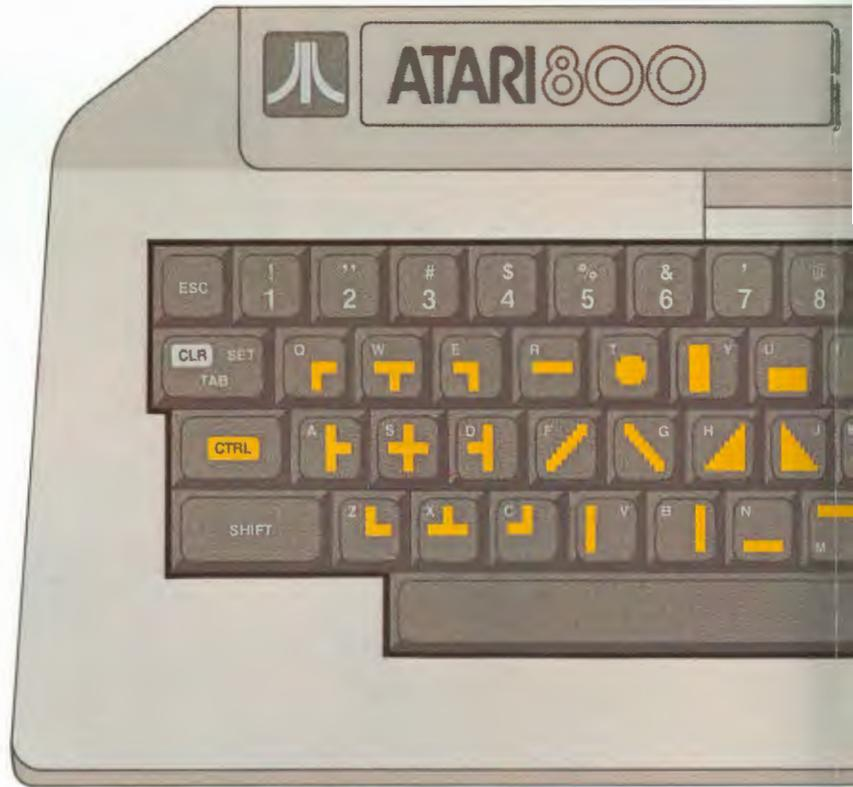
The **CTRL** (Control) key plays an important part in the screen editing functions; however, another key must be pressed while holding down the **CTRL** key for something to happen. The following list tells you what function occurs when the second key is pressed with the **CTRL** key.
