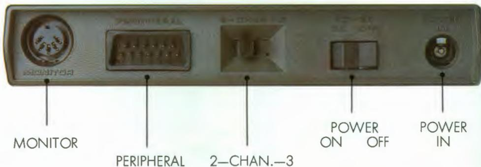
**8** Locate the AC Power Adapter that comes with the computer and plug the round end of the power adapter into the connector labeled **Power In** on the side of the computer console.
