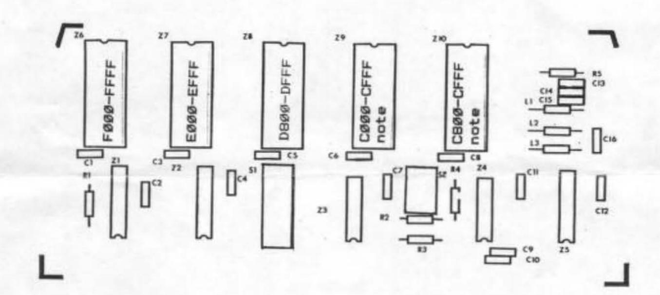
NOTE: Socket Z9 can be addressed as C000-C7FF or C000-CFFF depending on setting of switch two.
