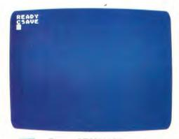
Press ADVANCE on the Program Recorder to wind the tape forward to the end of the last program recorded. Then wind the tape forward approximately 10 more counts (to make sure you do not record over another program). Now you are ready to record the next program. Make note of the tape count, then type cs AVE and press RETURN on the computer. You will hear two beeps (to remind you to press both PLAY and RECORD), then press RETURN again on the computer. The cassette will begin recording.
