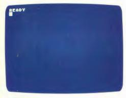
When the tape stops, your program has been loaded from the cassette to the computer. The television screen displays a READY prompt.
