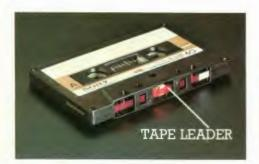
If you get an Error 143 or Error 138 message on your television screen during a loading procedure, your tape leader (the non-magnetized strip wound ahead of the actual recording tape) might be too long. As a result, the computer may be trying to read data where no data exists. Should this occur, rewind the tape to the beginning, then advance it approximately 10 counts. Now begin the loading procedure again.
