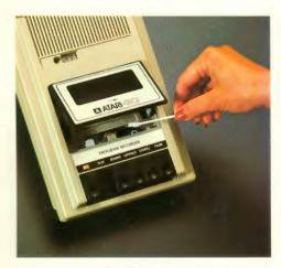
Wet a cotton swab with the cleaner and wipe the tape heads, capstan and pinch roller. Be careful not to leave bits of cotton behind. The capstan and pinch roller are best cleaned while they are turning. To do this, turn on your computer with the ATARI BASIC cartridge inserted, press STOP/EJ. to open the cassette door, then press PLAY on the recorder. Type CLOAD and press RETURN on the computer console. When the computer beeps, press RETURN again. The capstan will turn for about 20 seconds.
