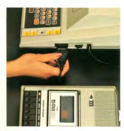
Plug the ATARI 410 Program Recorder data cord into the jack labeled PERIPHERAL on the right side of your ATARI Home Computer.
