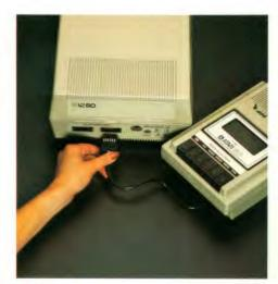
Plug the power cord that comes out of the back of the ATARI 410 Program Recorder into the wall outlet.
