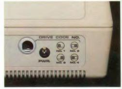
Using a pen or a screw-driver, set the Drive Code No. switches to match the Drive Code number shown in the diagrams. Set Disk Drive 2 to match DRIVE No. 2, etc.
