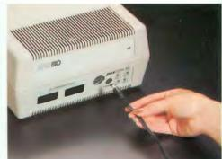
Plug one end of the I/O Data Cord into the jack on the side of the computer console marked PERIPHERAL. Plug the other end into one of the jacks marked I/O CONNECTORS on the back of the disk drive. If you have an ATARI 410 Program Recorder, plug it into the remaining I/O CONNECTOR jack.
