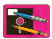
Do not write on your diskettes with a pencil or a ball-point pen. The sharp point of a pencil or ball-point pen can score the surface of the diskette. Use a felt-tip pen to mark the diskette label or write on the label before you put it on the diskette.
