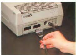
Turn on the disk drive. When the red BUSY light goes off, open the door to the disk drive by pushing the rectangular button to the left of the ATARI 810 label.
