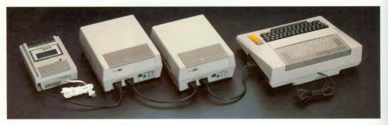
If you have more than one ATARI 810 Disk Drive, you must set two small switches on each disk drive so that the computer knows which drive you are referring to in your programs or commands. You must always have one disk drive in the chain set as Drive 1.
