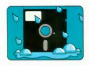
Never wet or wash a diskette. Use a soft brush or compressed air from a spray can to remove any dust from the surface.
