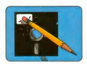
Do not use pencil erasers on diskette labels. Eraser dust is abrasive and will damage the diskette.
