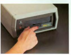
When you turn on the computer, DOS loads automatically. If you turn up the volume on your TV set while DOS is loading, you'll hear a series of beeps. This is perfectly normal and lets you know DOS is being loaded into the computer.
