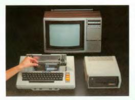
Remove the ATARI Master Diskette II from its protective sleeve and insert it into the disk drive with the label facing up. Then close the door.
