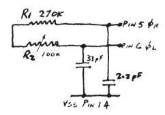
Set frequency of S1 to 3.781Khz + 1% by adjusting R2. This gives 121KHz data bursts at serial output (Pin 15).
