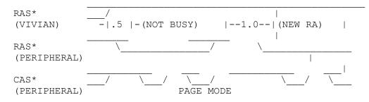
PERIPHERAL AUTOMATICALLY CHANGES THE CAS\* TIMING FROM NEGATIVE CLOCK TO POSITIVE CLOCK AS SYSTEM SWITCHES FROM VIVIAN TO THE PERIPHERAL.
